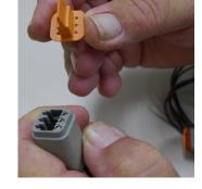
3. Using small screw driver remove wedge lock from connector.
