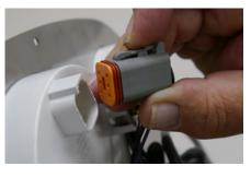
1. Remove 6 pin Deutsch by depressing release tab and pulling outward.
