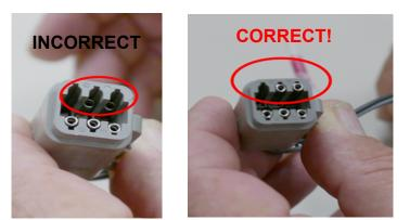
5. Install red power wire in pin location 1 or 6. Install black ground wire in pin location 2 or 5. Visually inspect wire pin for proper installation. Reinstall wedge lock and weather gasket. Reinstall connector to gauge.
